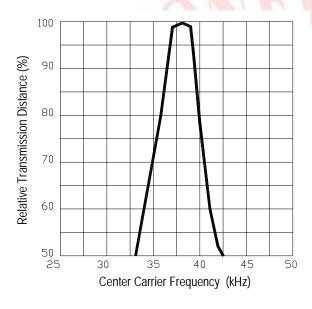
Fig.-11 Relative Transmission Distance vs. Center Carrier Frequency IRM-H640/TR2
