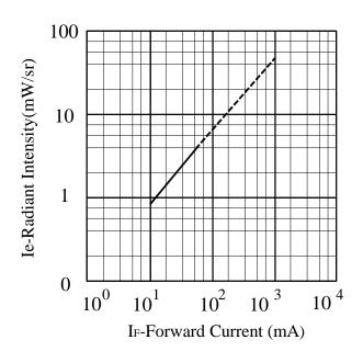
Fig.6 Relative Radiant Intensity vs.
