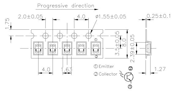
Note: The tolerances unless mentioned are ±0.1, unit=mm
