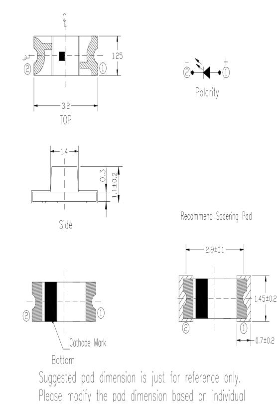
Note: Tolerances unless mentioned ±0.1mm. Unit = mm
